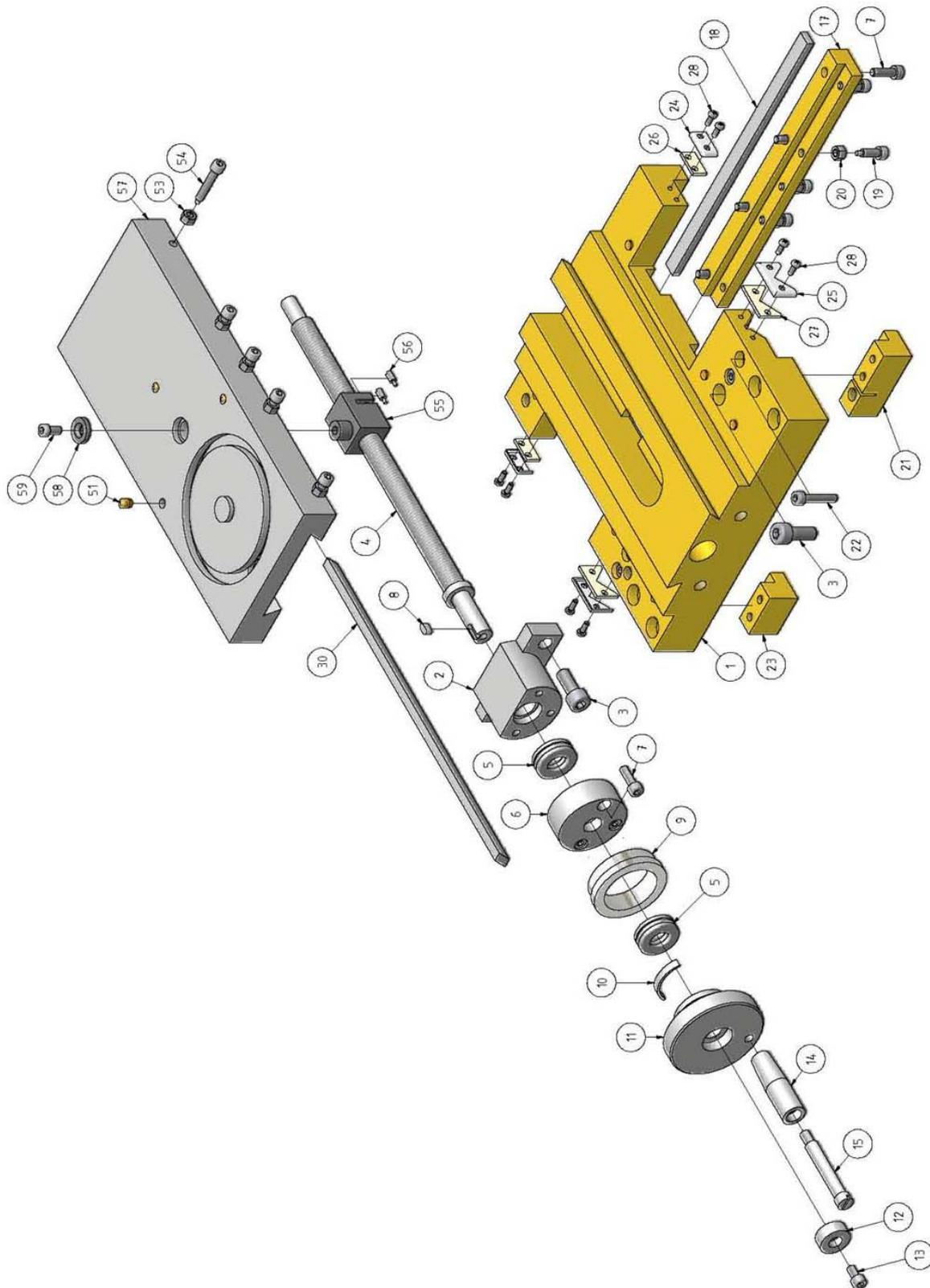
Abb.8-2: Planschlitten - Cross slide
