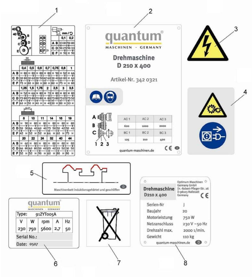
Abb.8-13: Maschinenschilder - Machine labels
