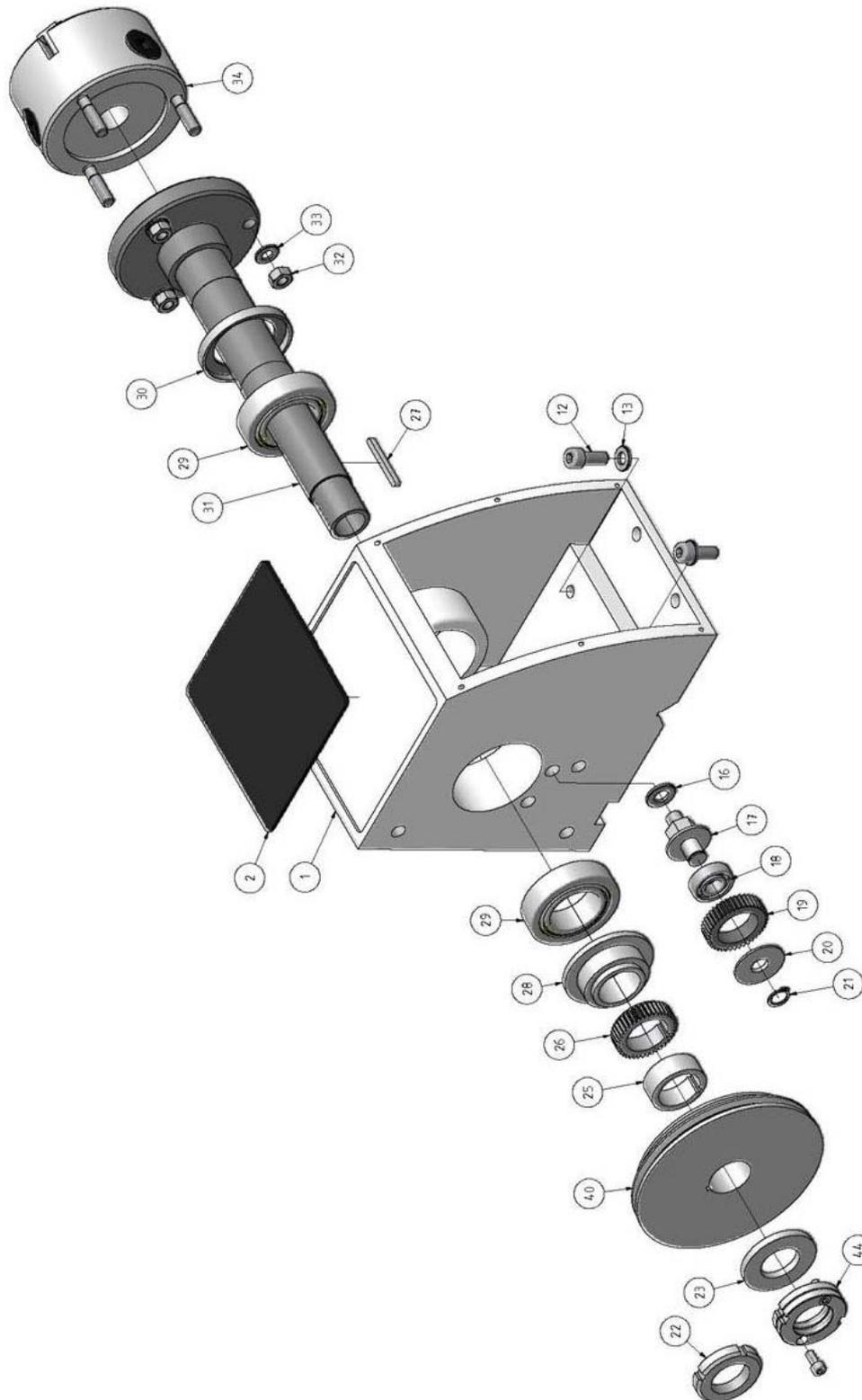
Abb. 8-8: Spindelstock - Headstock
