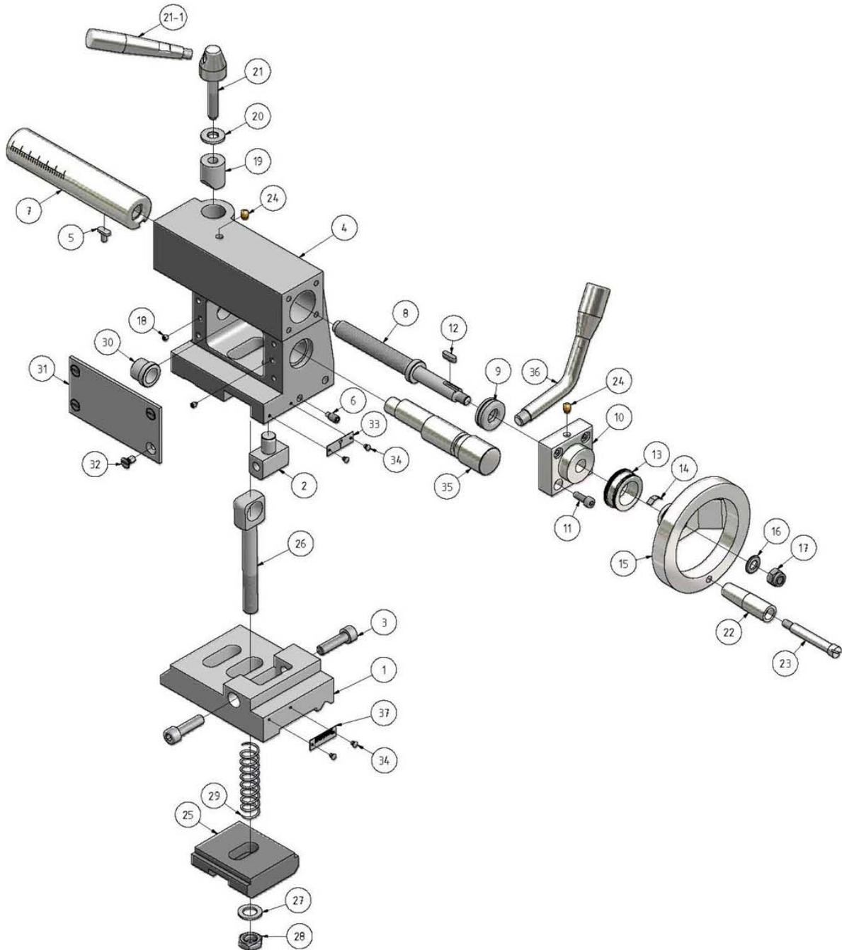
Abb. 8-6: Reitstock ab Baujahr 2008 - Tailstock starting from year of construction 2008
