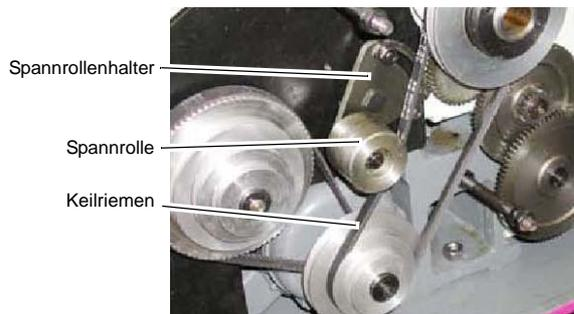
Abb. 4-7: Spannrolle D 210 x 400
