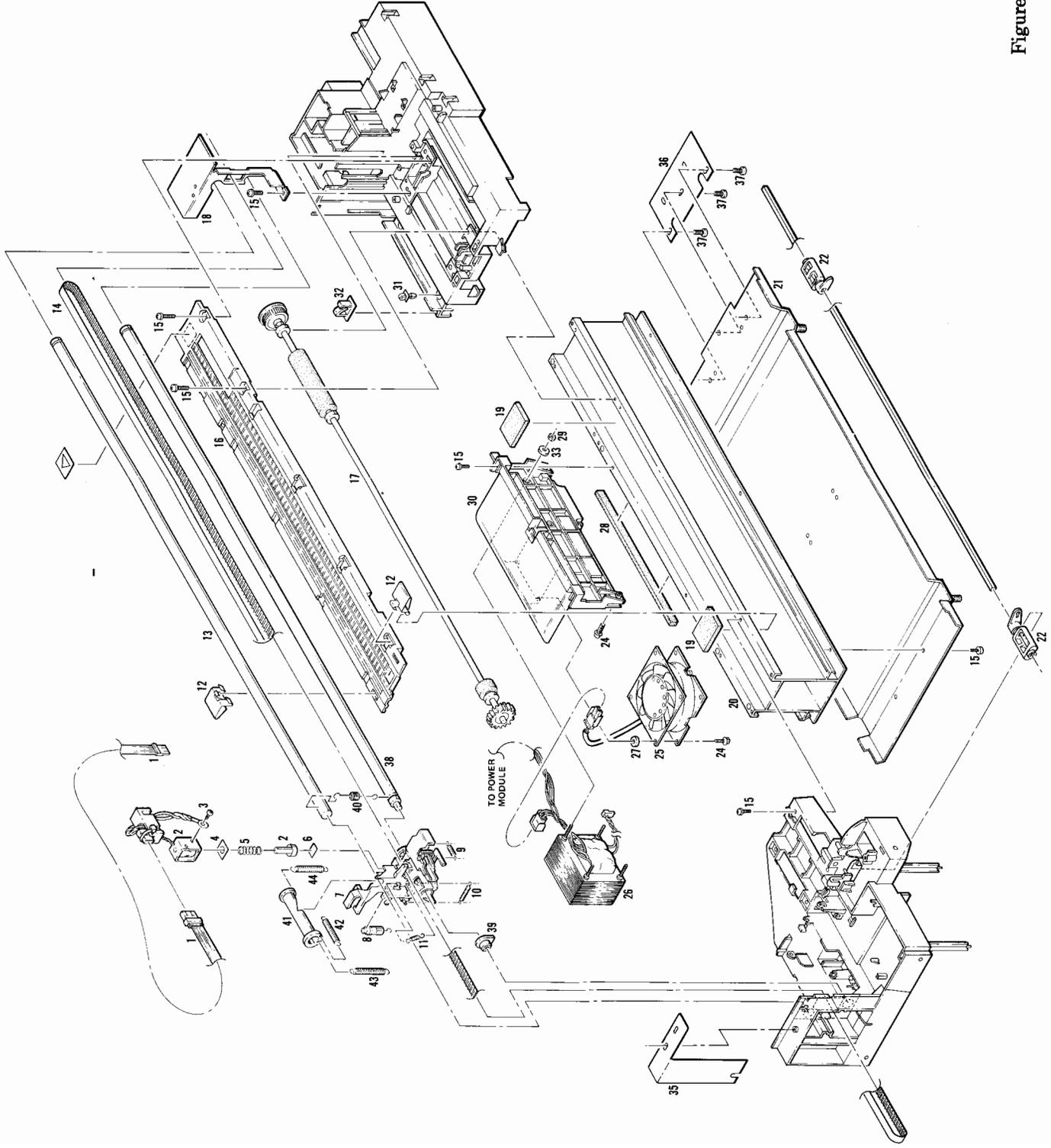
Figure 8-3. Center Chassis Assembly, Illustrated Parts Breakout
